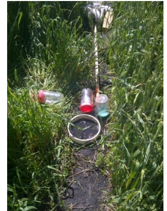
Figure 13. Water infiltration test with a 7" ring.
