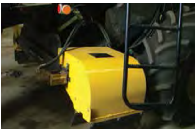
Photo 7.14 a) Chaff diverter cyclone for conveying chaff and extra spreaders for straw; b) Thick chaff on the wheeltrack diverted by using this system by the late Owen Brownky (Source: Glen Riethmuller DAFWA).
