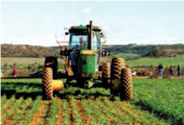
Photo 4.4 Cotton reels have been used to extend the axles to 3 m on this JD4250MFWD (Source: DAFWA Bulletin 4607 Webb et al 2004).
