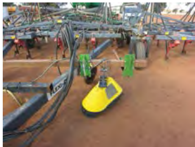
Photo 4.18 Spraying Shield and straw discs on the wheel tracks to assist with weed control in the wheel tracks (Source: Glen Riethmuller, DAFWA).
