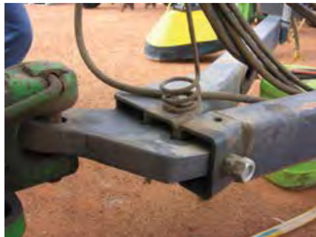
Photo 7.2 The late Owen Brownley's offset hitch (Source: Glen Riethmuller, DAFWA).
