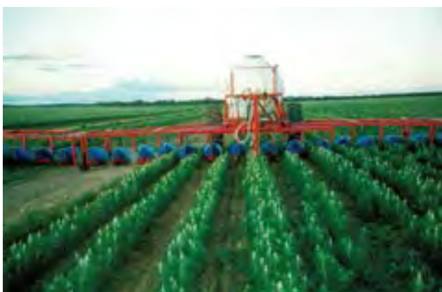
Photo 7.10 Self steering shields made from materials on farm (Source: Paul Blackwell, DAFWA).
