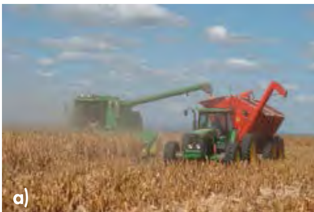
Photo 4.12 a) Catching hopper and cross auger on the chaser bin to allow unloading from the wheel tracks; b) Catching hopper on the chaser bin (Source: Rob Taylor).
