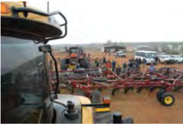
Photo 8.24 Carsons machinery lined up showing most wheels on 3 m and some seeder wheels at 4 m (Source: Stephen Davies, DAFWA).
