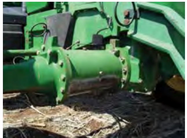
Photo 4.7 C&C Machining & Engineering axle modification spacer on certain John Deere tractors (Source, Tim Neale precisionagriculture.com.au).
