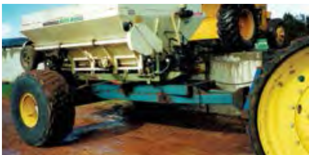
Photo 4.11 The spreader is mounted on an old truck axle extended to 3 m. Modifications to vehicle axles may require risk assessment on farm and recertification for road use (Source: Webb et al. 2004).
