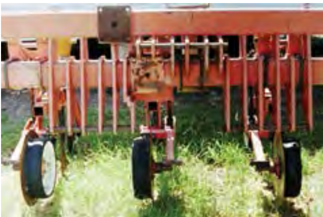
Photo 7.5 Multi-hitch for three point linkage (Source: Western Australian Agriculture Authority).
