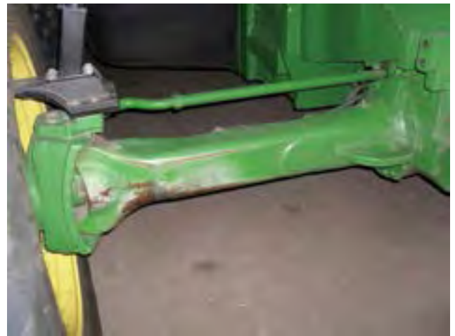
Photo 4.6 C&C Machining & Engineering axle modification (Source: Tim Neale, precisionagriculture.com.au).
