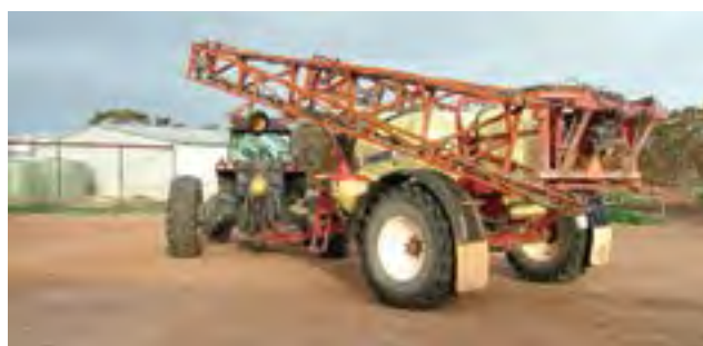
Photo 8.3 Sprayer with extended axels to 3 m (Source: Western Australian Agriculture Authority).
