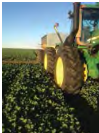
Photo 8.6 Marshall spreader and 9300 JD Tractor on 3 m wheel tracks (Source: Paddy Barber).
