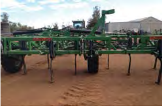
Photo 8.16 Deep ripper with tines moved from behind the wheel tracks (Source: Brady Green).
