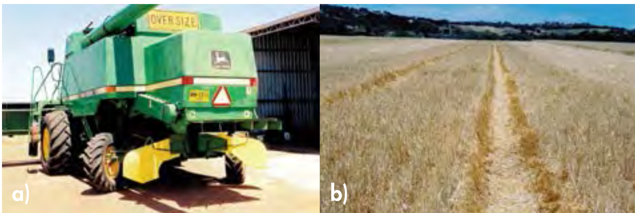
Photo 7.13 a) Farmer designed and engineered chaff diverters; b) Chaff diverted into the wheeltrack by the chaff diverters from a three tonne crop (Source: Webb et al 2004).
