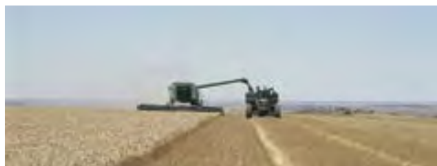
Photo 4.13 Auger extended to allow unloading on the wheel tracks (Source: DAFWA Webb et al 2004).
