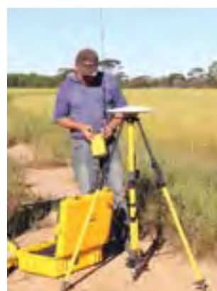
Photo 5.5 (left) Setting up a Trimble base station at GSARI Katanning (Source: Glen Riethmuller, DAFWA).
