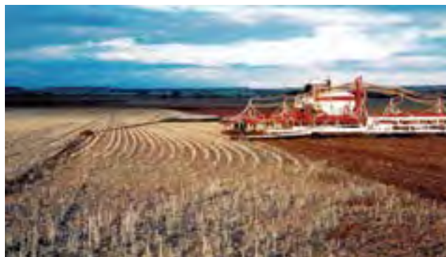
Photo 5.2 One marker arm on a 60 foot seeder, seeding round and round (Source: Western Australian Agriculture Authority).
