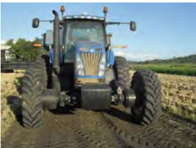
Photo 4.5 New Holland Front Wheel Assist on 3 m with cotton reels (Source: Tim Neale, precisionagriculture.com.au).
