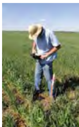
Photo 3.3 Handheld penetrometer with pressure gauge and GPS logger attached (Source: Paul Blackwell, DAFWA).
