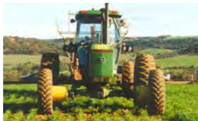
Photo 8.20 Moffats original spraying tractor axle extended by cotton reels (Source: Webb et al 2004).
