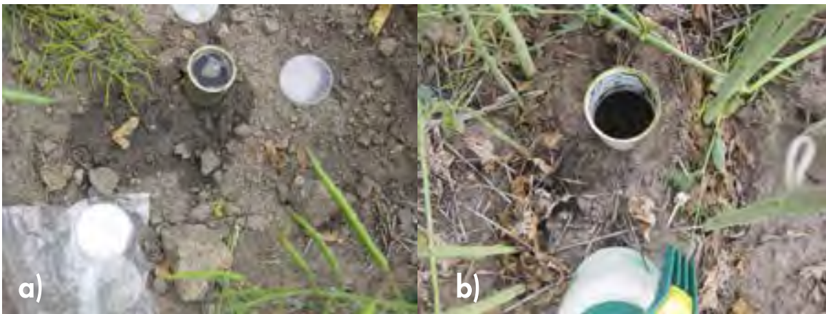
Photo 8.12 a) Water infiltration on the wheel track and b) Faster water infiltration rate off the wheel track.
